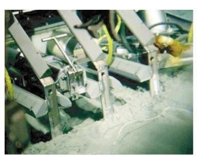
*FIGURE 2-6* The starboard side of the HUGO junction box on Loihi seamount off Hawaii. Experiments are installed and repaired using the Pisces V submersible. SOURCE: Fred Duennebier, University of Hawaii.
