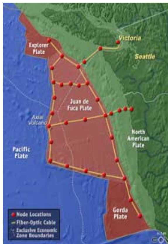
Figure 1. Bathymetric map showing the layout for NEPTUNE. The yellow line and red dots denote the backbone cable and locations of the seafloor science nodes, respectively. The white line is the approximate boundary of the US and Canadian Exclusive Economic Zones.
