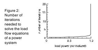
While convergence of the software and stability of the system are not exactly equivalent, they are strongly related. Provided power transfer is kept at or below about 95% of the theoretical peak value, stable operation should result.
