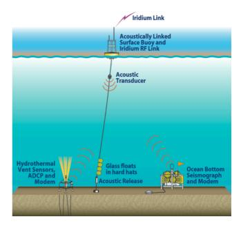
Fig. 1. Conceptual drawing of an acoustically-linked observatory.
