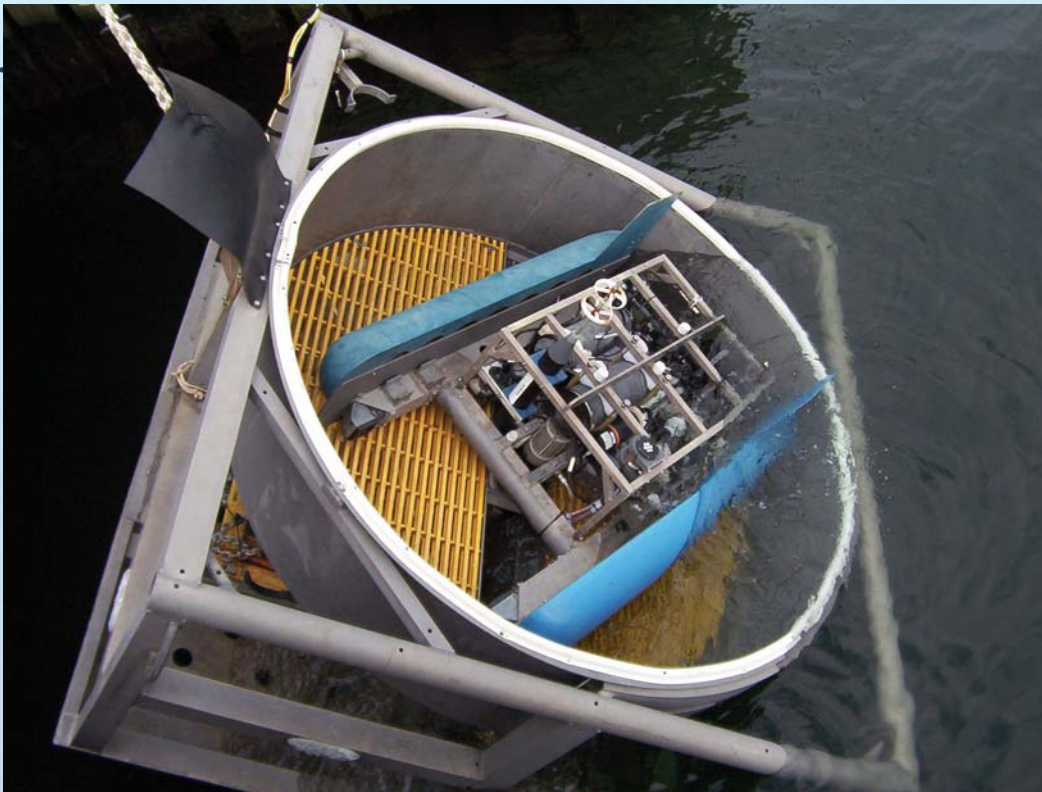
Deployment of the Autonomous Vertically Profiling Plankton Observatory (AVPPO) at the Martha's Vineyard Observatory. The AVPPO is an underwater winch and buoyant sensor platform containing bio-optical (irradiance, ac-9, OBS), physical (turbulence, ADCP), chemical ( O_2 , nitrate) and biological (Video Plankton Recorder, fluorometer) sensors. Profiles are made to the air-water interface once per hour while data are telemetered to shore in real-time. For more information, go to http://4dgeo.who.edu/vpr .
